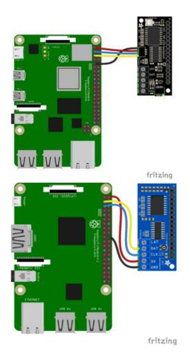
Pi 3V to backpack VIN Pi GND to backpack GND. Pi SCL to backpack CLK. Pi SDA to backpack DAT.
