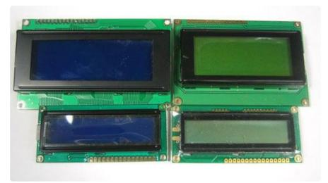
This backpack will work with any 'standard'/'classic' character LCD. It does not work with graphic LCDs. Character LCDs come in sizes ranging from 8x1 (8 characters, one line) to 40x4 (40 characters, four lines). The backpack will also only fit LCDs that have a single line of pins at the top, not the ones that have a 2x10 or 2x8 connector on the side. Those are much rarer these days but just keep a look out for that!
