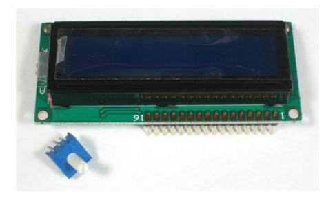
The easiest way we know of doing this is sticking the header into a breadboard and then sitting the LCD on top while soldering. this keeps it steady.
