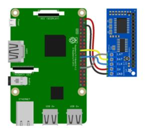
Pi 3V to backpack VIN Pi GND to backpack GND. Pi SCK to backpack CLK. Pi MOSI to backpack DAT. Pi GPIO5 to backpack LAT.
