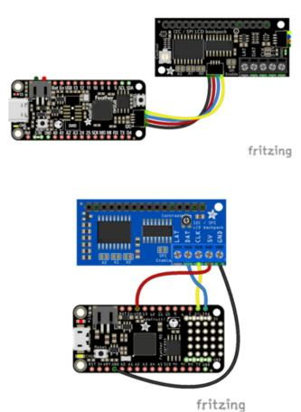
Board 3V to backpack VIN Board GND to backpack GND Board SCL to backpack CLK Board SDA to backpack DAT If using the original version of the backpack:
