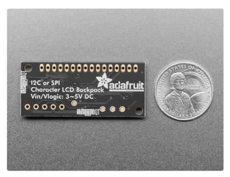
By using simple I2C and SPI input/output expanders we have reduced the number of pins, while still making it easy to interface with the LCD. Only 2 pins are needed for I2C, 3 for SPI. For Arduino and CircuitPython/Python users, we provide an easy-to-use library that is backwards compatible with projects using the '6 pin' wiring.
