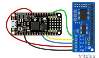
Board 3V to backpack VIN Board GND to backpack GND. Board SCK to backpack CLK. Board MOSI to backpack DAT. Board D5 to backpack LAT. If using the original version of the backpack:
