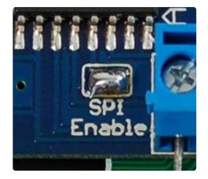
This will switch the backpack over to SPI mode instead of I2C. If you want to go back to I2C, use wick or a solder sucker to remove the jumper
